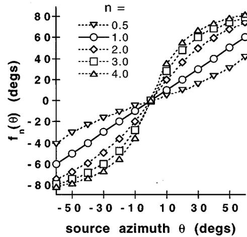
FIG. 1. Plot of the family of functions  $f_n(\theta)$  used to transform auditory localization cues. With this transformation, a source from azimuth  $\theta$  was synthesized using the HRTF that normally corresponded to the position  $f_n(\theta)$ .
