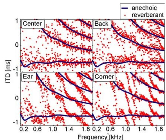
**Fig. 5** ITDs as a function of frequency in the anechoic and reverberant conditions for source at  $90^\circ$  1 m.
