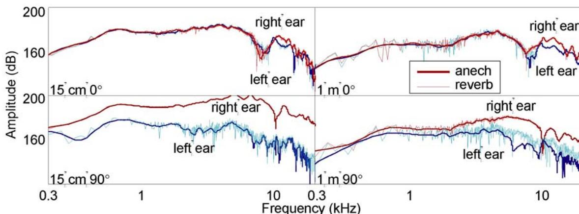
Fig. 2 Anechoic and reverberant magnitude spectra at four source positions with KEMAR in center of room.
