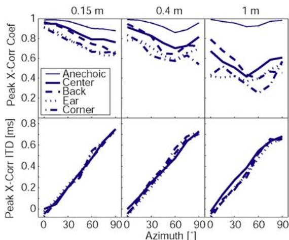
**Fig. 4** The peak value in the cross-correlation function within  $\pm 1$  ms range and the corresponding ITD.
